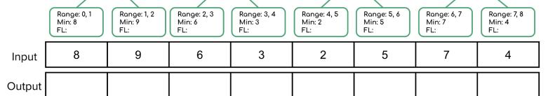
Second pass: fill out the *FL* ("from left") field starting from the top down to the leaf nodes to represent the minimum value of the *prefix* of this subproblem's range, that is, the min of everything to the *left* of this node. This can calculated with the following expressions:
